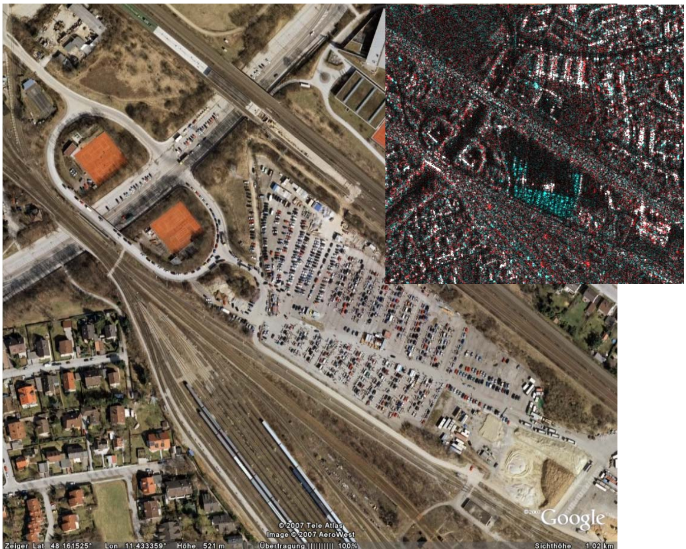
Figure 1. Example of change detection is presented as RGB image in the upper right part (R: Saturday 7-7-2007, B: Tuesday 26-6-2007) for TerraSAR-X (StripMap, HH, descending mode, resolution azxrg 3mx1.2m) over Munich. We can see clearly how the car-park is half filled on the working day (blue color) in comparison with a weekend. Google image is used as a background.
